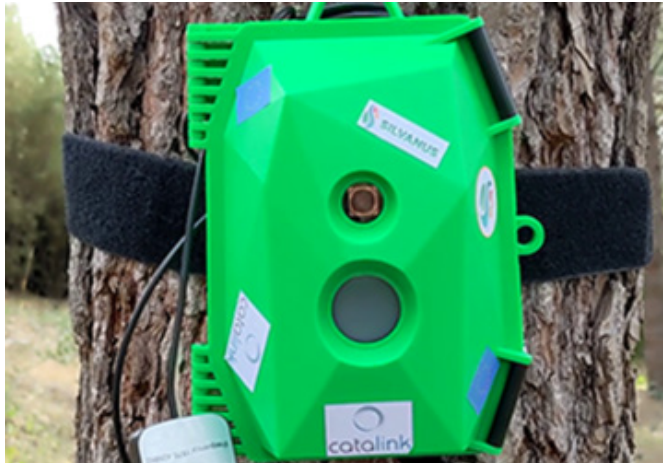
Figure 22. IoT element designed to detect a wildfire
