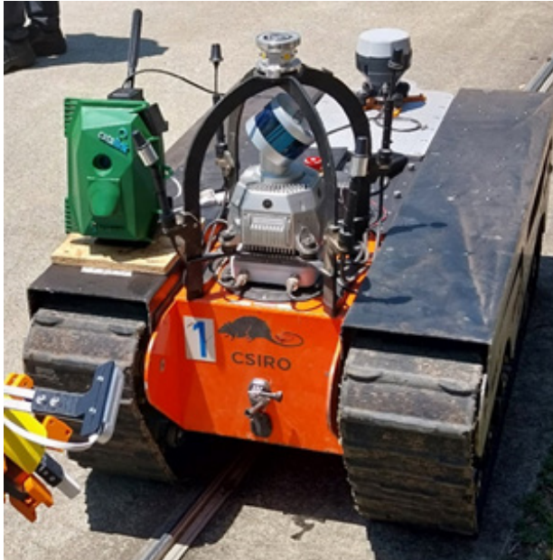
Figure 29. Robot integrated with a smoke detector, LIDAR and a geo-localiser
