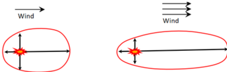
Figure 8. Influence of wind speed on fire shape
