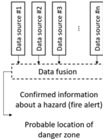
Figure 38. The general idea of data fusion in the forest fire alert system
