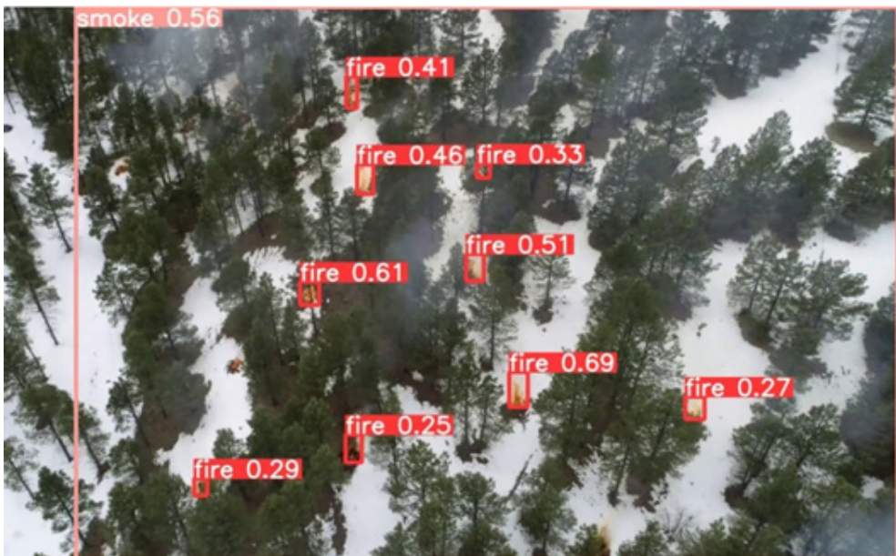
Figure 22. Visualisation of danger zone (smoke) and hotspots after the use of fire detection at the Edge (the view from a UAVs)
