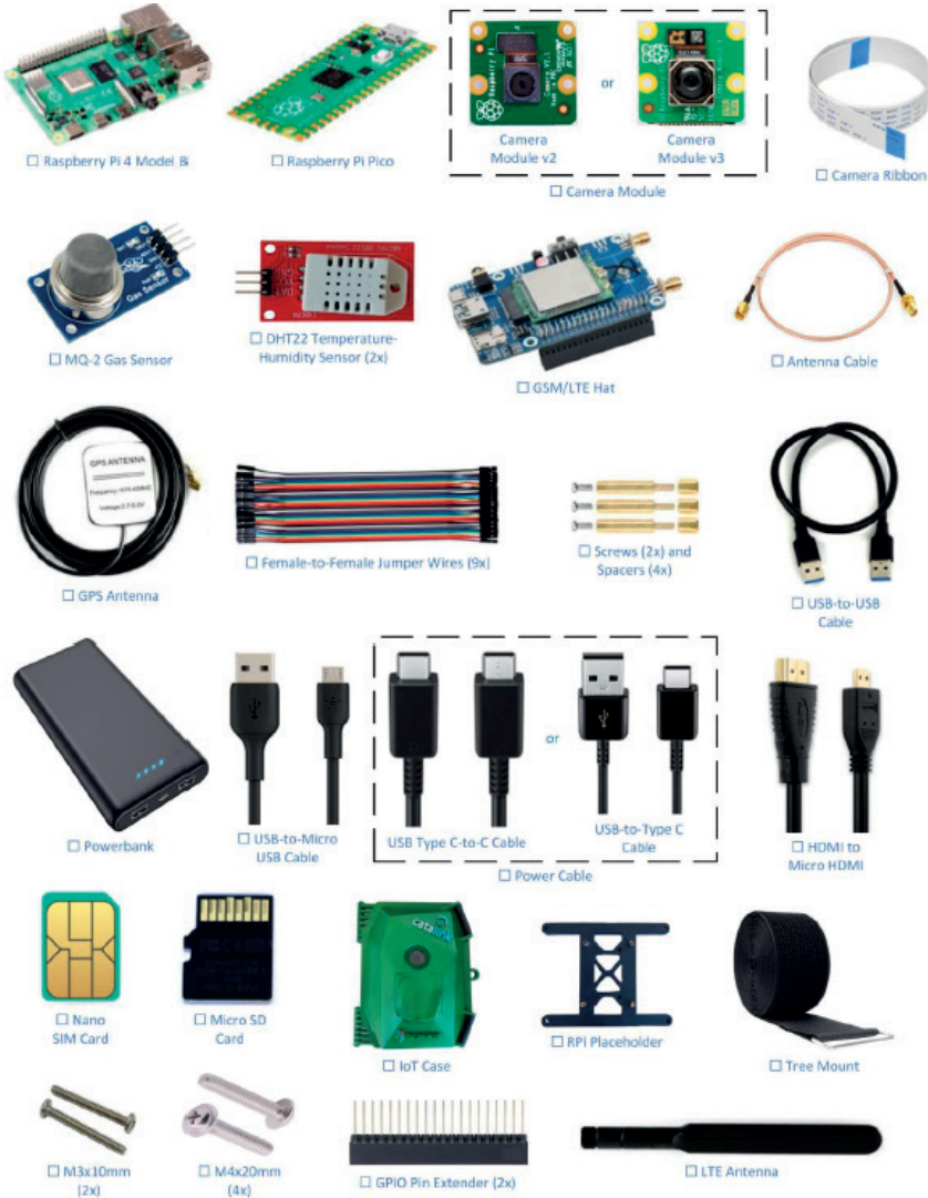
Figure 7. IoT items collected for one device to detect a wildfire
