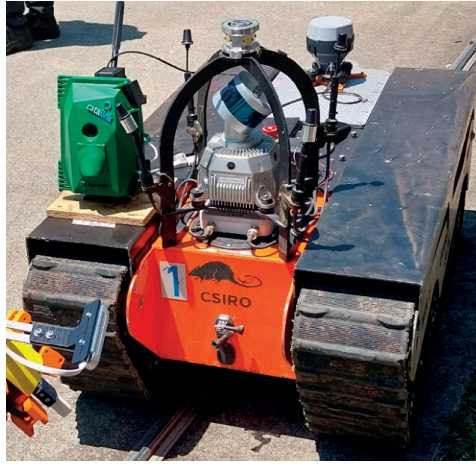
Figure 31. Robot integrated with a smoke detector, LIDAR and geo-localiser
