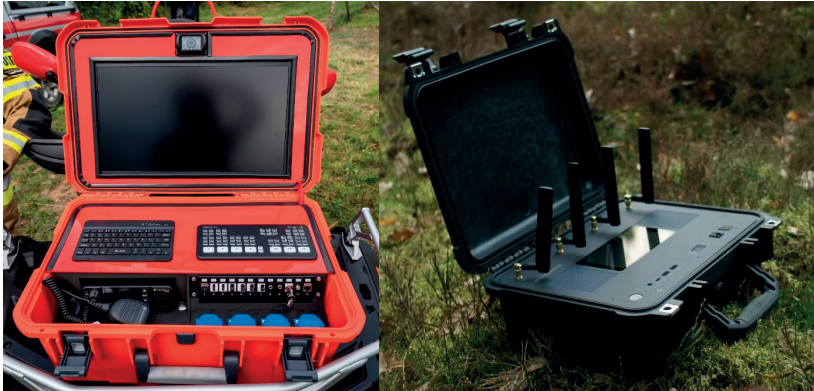
Figure 28. Overview of selected systems for real-time wireless video transmission from a UAV. On the left – Mobile Command Centre (RPASAR), on the right – ACO Streamer 4K LTEA (ACO Solutions) Source: (RPASAR, 2022; Fellner, 2023)
