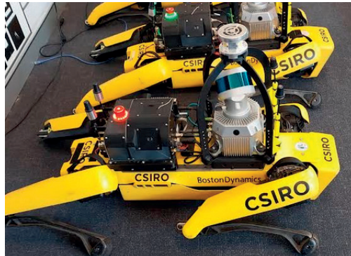
Figure 32. Walking robot integrated with LIDAR and geo-localiser
