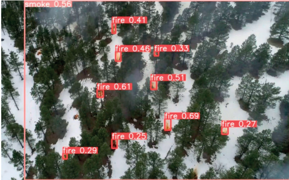
Figure 11. Visualisation of danger zone (smoke) and hotspots using fire detection at the Edge (view from a drone)
