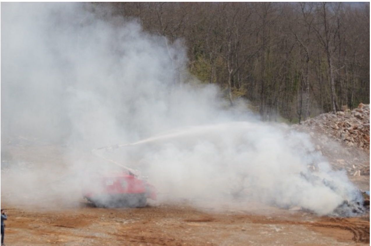
Figure 25 - Water spray evaluation for fire suppression
