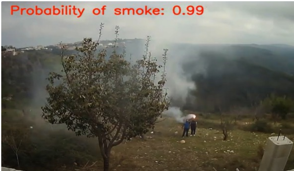
Figure 120 – Frame extracted from the lightning torch test video analysed by CATALINK algorithm
