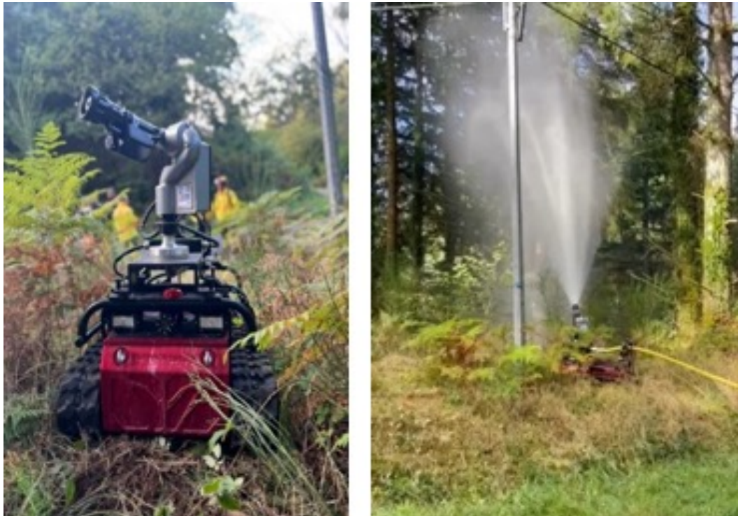
Figure 85 - Demonstration of ground robots for testing fire spray for suppression
