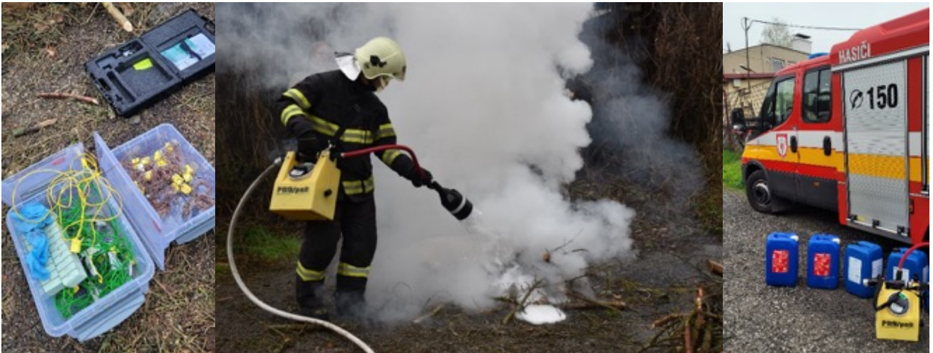
Figure 42 – Testing the efficiency of extinguishing substances friendly to wildland environment
