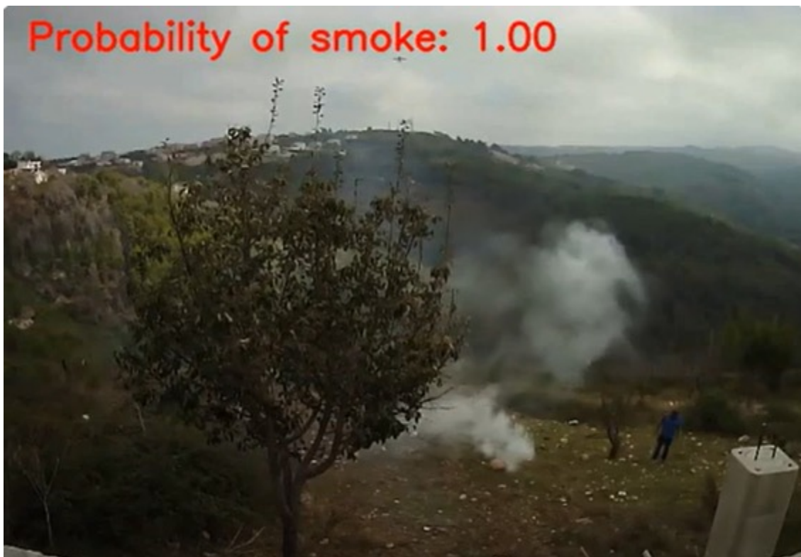
Figure 121 – Frame extracted from the video of the test with the smoke bomb analysed by CATALINK algorithm
