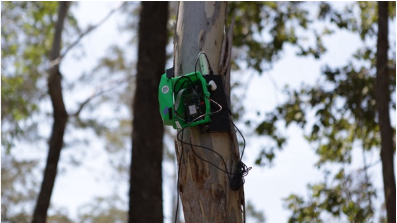
Figure 164 - Deployment of in-situ devices on the forest for smoke and fire detection
