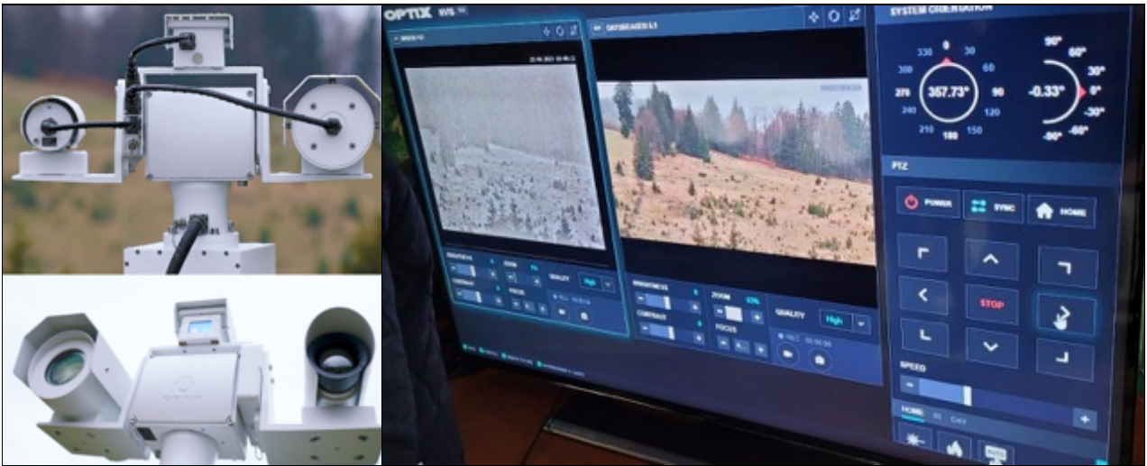
Figure 48 – Smoke/fire detection by camera monitoring system
