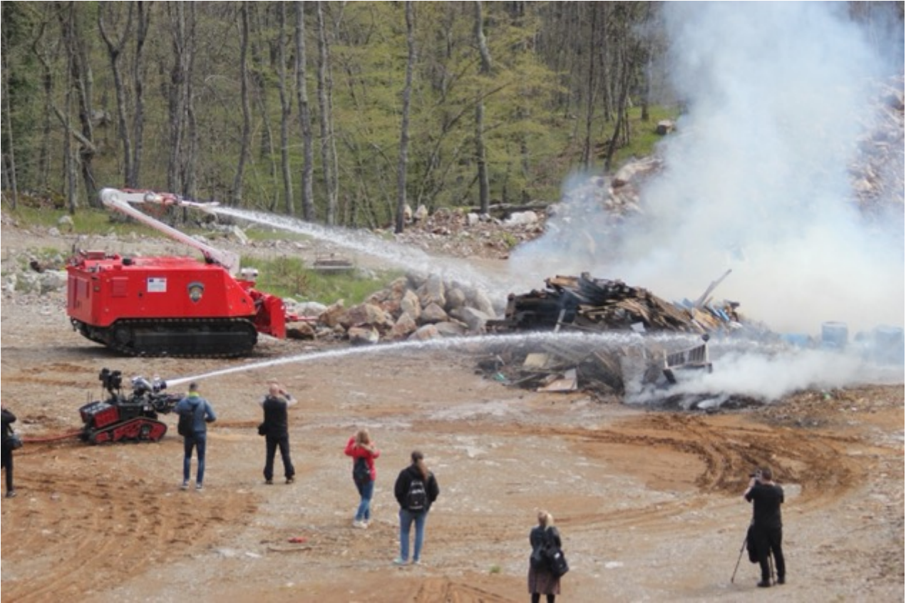
Figure 26 - Fire suppression with two different ground robots and performance assessment
