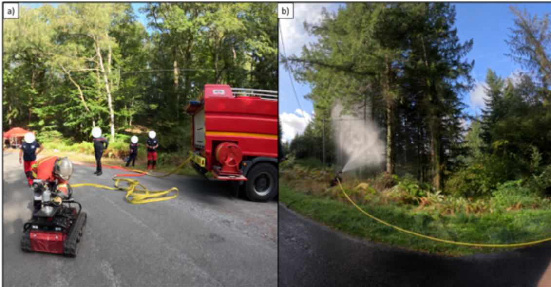
Figure 78 - Installation of fire hose to the ground robot and testing of water spray capacity from the ground robot
