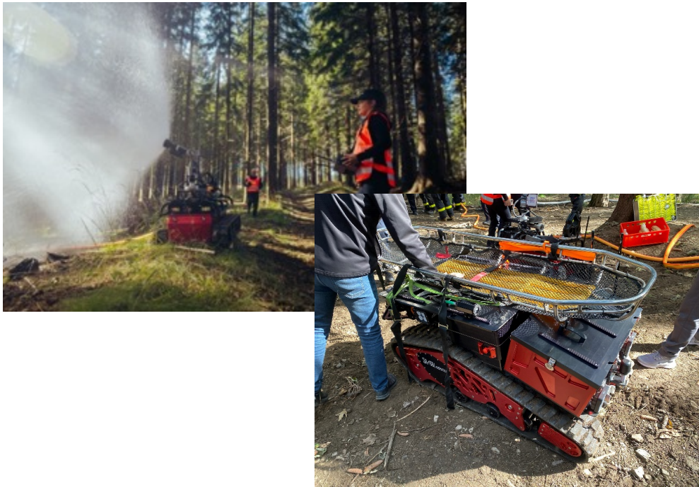
Figure 104 - Ground robots under demonstration for fire suppression
