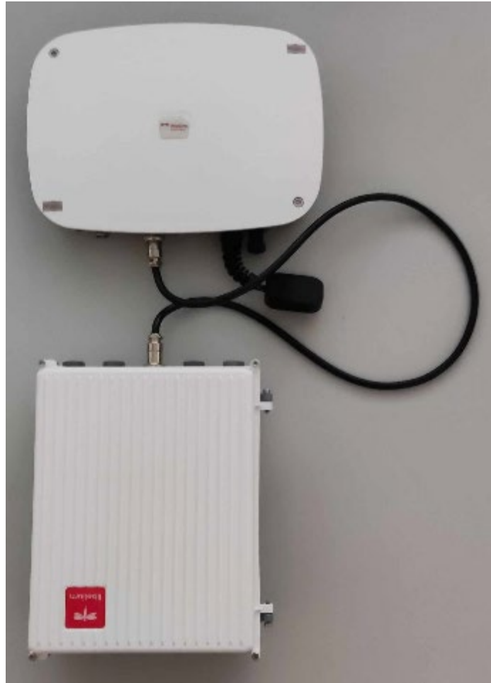
Figure 107: Smart Spot - IoT device for environmental parameter sensing
