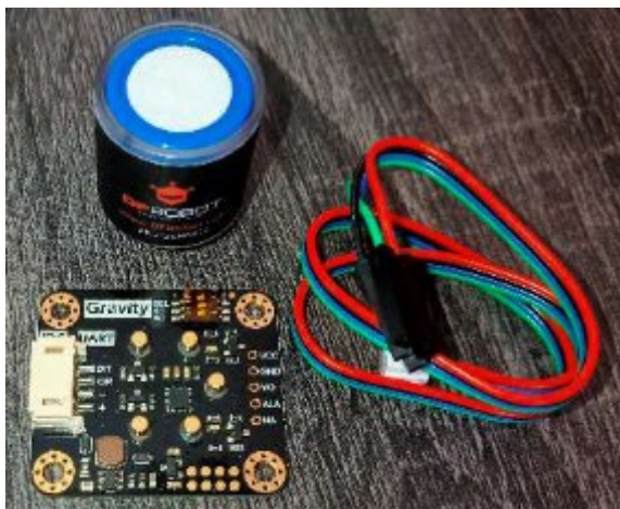
Figure 94: Gas Sensor Components
