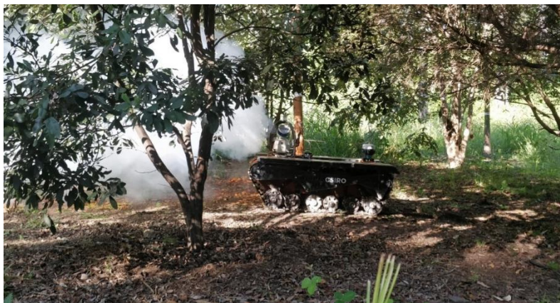
Figure 55. The CSIRO UGV platform autonomously navigating in complex, natural terrain in the presence of (artificial) smoke, during a simulated mid-fire scouting operation.
