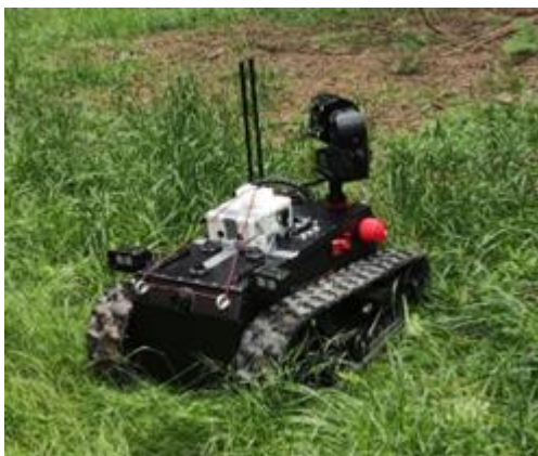
Figure 34. Installation of UP9b on an UGV.
