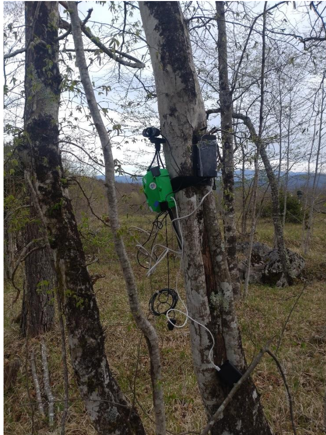
Figure 29. UP4a IoT device connected to the MESH in the Sky node.
