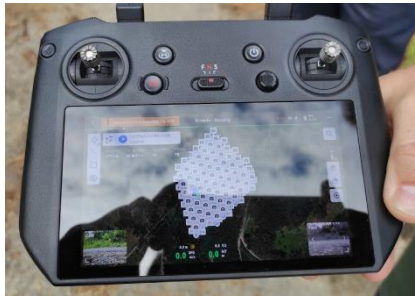
c) KML-formatted drone route prepared and loaded to the drone controller before the flight.
