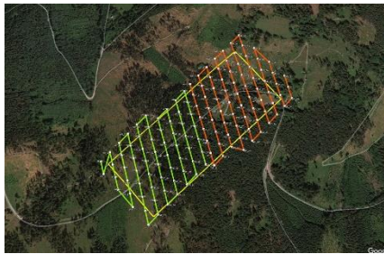
b) Trajectories of optimal planned drone routes in KML-format precomputed and prepared for drone pilots.
