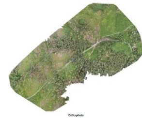
d) Result of the drone image stitching from two independent drone flights.
