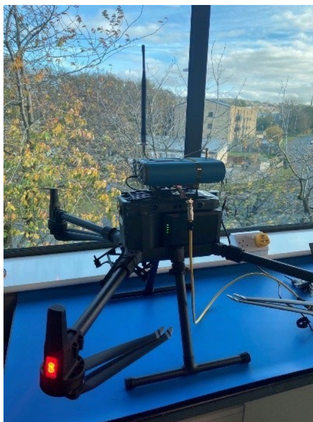
Figure 4 UAV with integrated Mesh in the Sky node during laboratory testing
