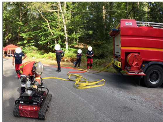
Figure 12: Installation of fire hose to the ground robot
