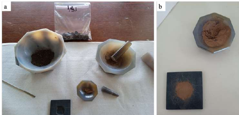
Figure 10. Preparation of the soils for the XRD analyses. a) Use of agate mortars in multiple sizes in order to pulverize the soil and b) the produced powder is placed in the sample holder.
