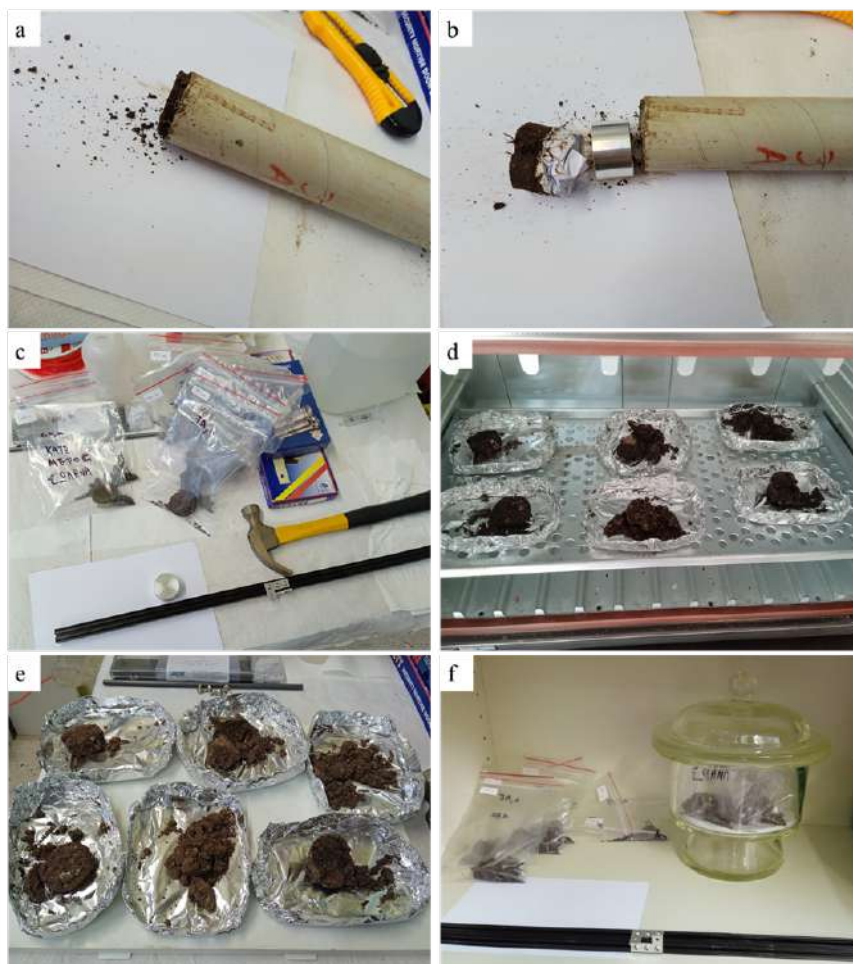
Figure 8. a) Hollow plastic tube, filled with the core sample, b) removing the core sample with a piston and dividing it in every 2 cm, c) storage of each sample, d) dehydration at 50°C, e) dehydrated samples, and e) final storage of the dehydrated samples in the desiccator.
