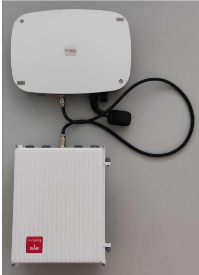
**Figure 107: Smart Spot - IoT device for environmental parameter sensing**
