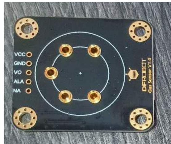
Figure 95: Gas Detection Sensor
