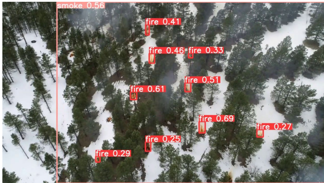
Figure 20 – Fire and smoke detection using real time video (video extract)
