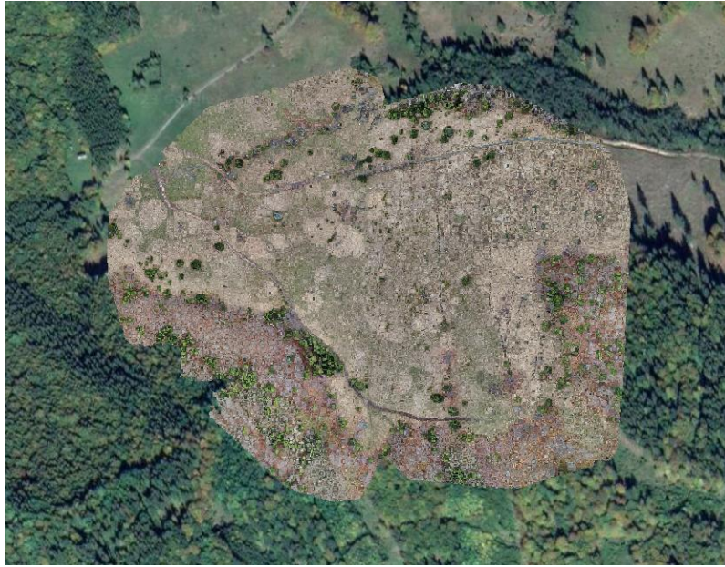
Figure 29: Orthophomap created from successive pictures taken by drone during the Slovak pilot event
