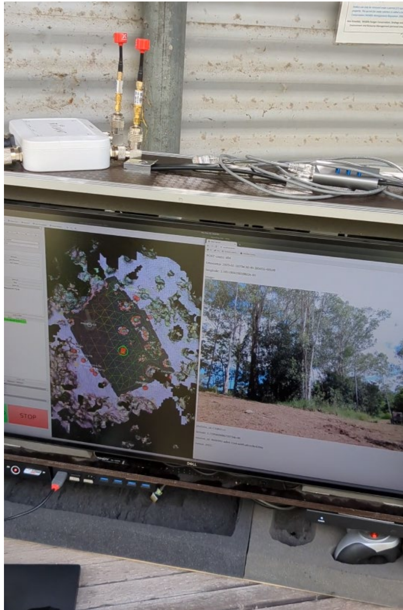
Figure 14 - Base station showing command interface (left), map plan view (middle) and front camera view (right). The communications link is above the screen, and teleoperations controller shown bottom right.
