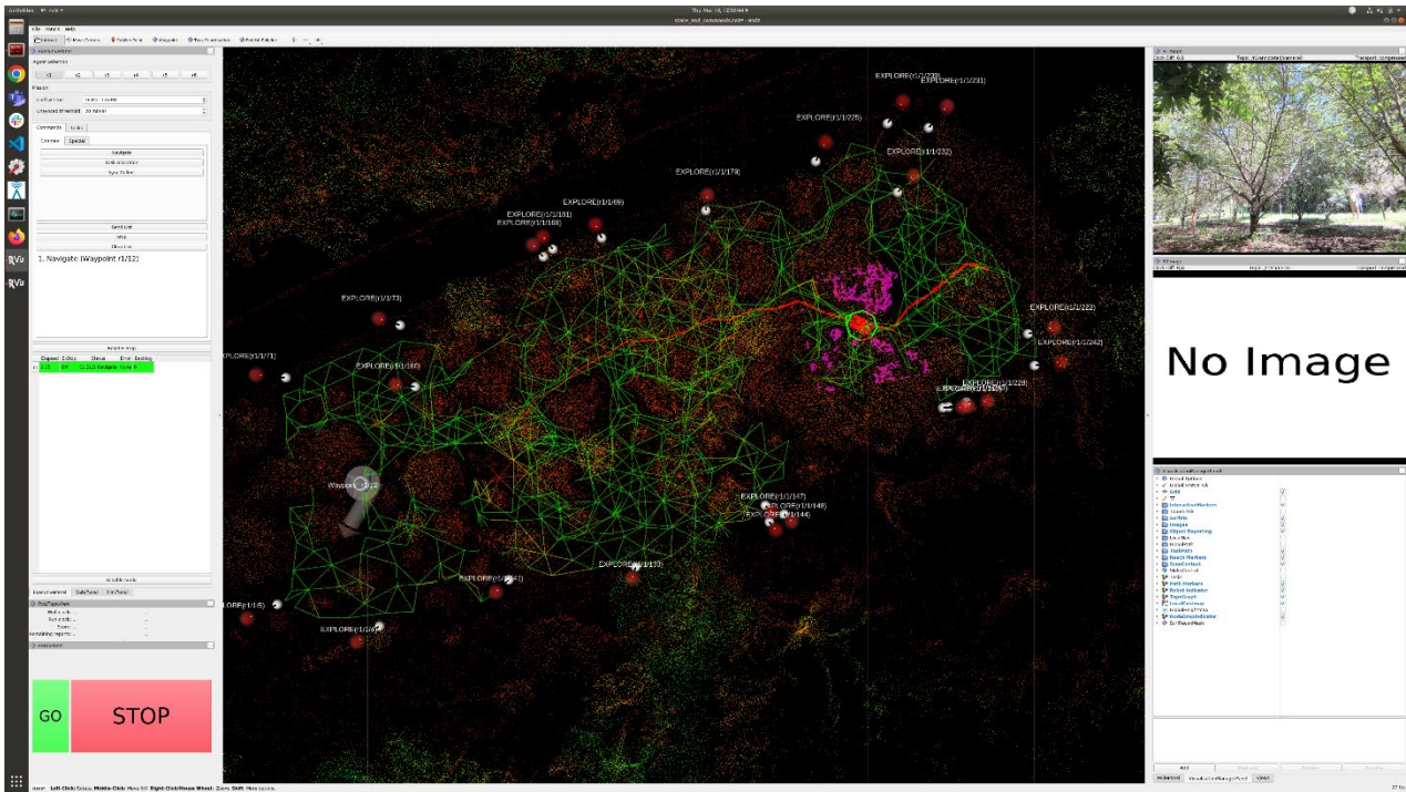
Figure 20 - Basestation showing autonomous return journey (red path) from frontline (right) back to human-safe location (grey disk).
