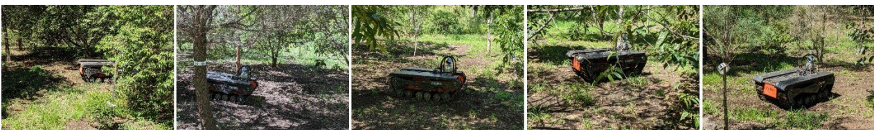
Figure 19 - Return traversal of the UGV was fully autonomous and without any back tracking, due to the outbound acquired map.
