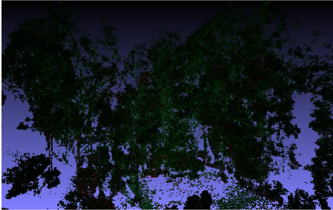
Figure 9 - Removing all points where r+g > 0.3 , using the raysplit colour command leaves primarily foliage and ground.
