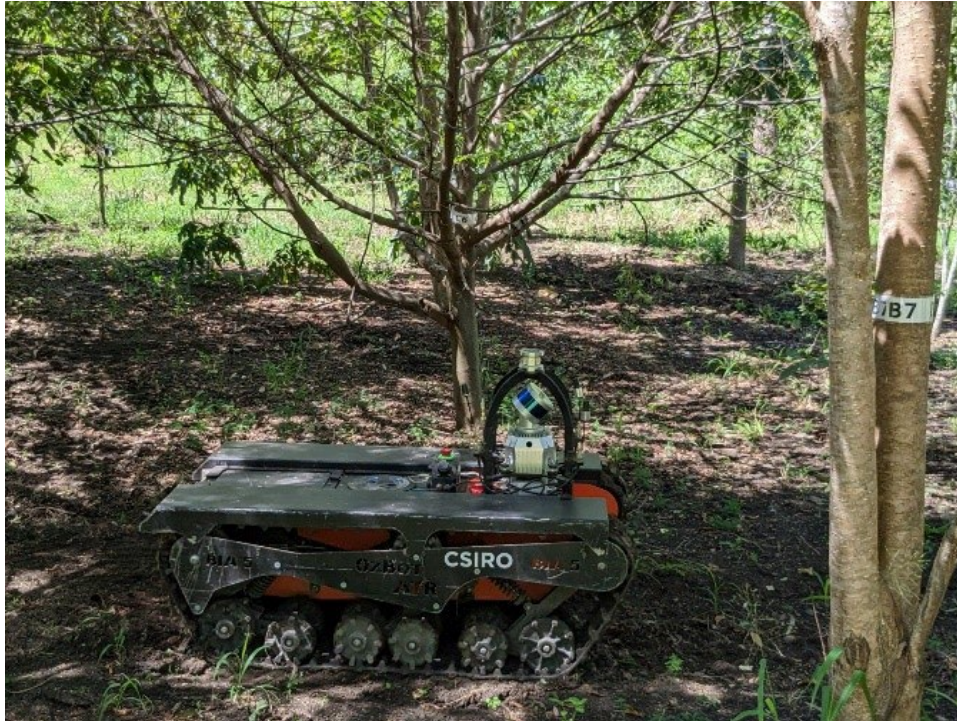
Figure 13 - The tree, scrub and grass environment used in this demonstration. The sensor and navigation payload can be seen on the right side of the ATR.
