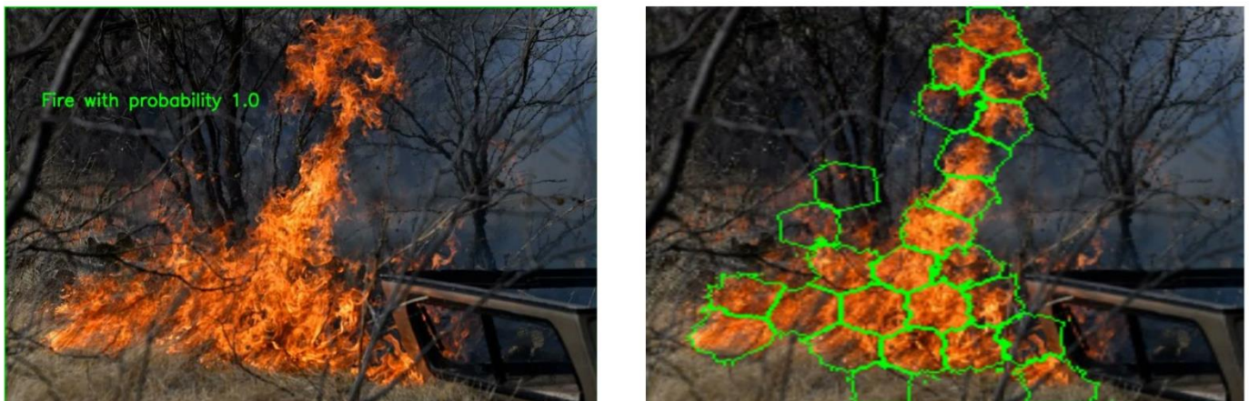
Figure 24: (left) Example output of the fire binary classification model (with fire probability = 1) and (right) an output example of the fire superpixel localisation algorithm
