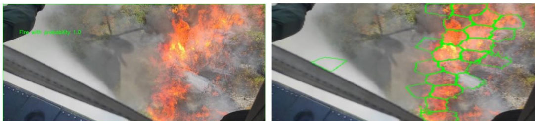
Figure 44 - (left) Example output of the fire binary classification model and (right) an output example of the fire superpixel localisation algorithm.
