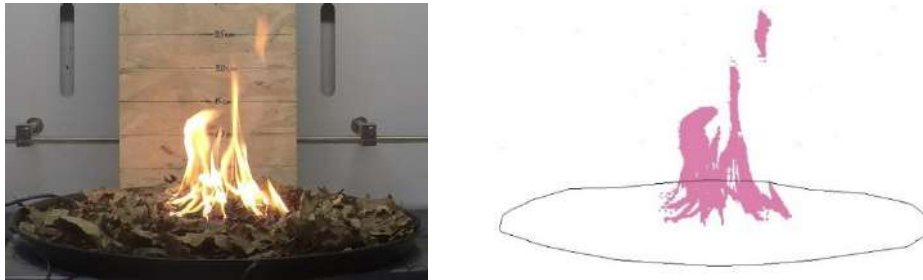
Figure 47 Flame area during the fire test 1 in time of 20 s
